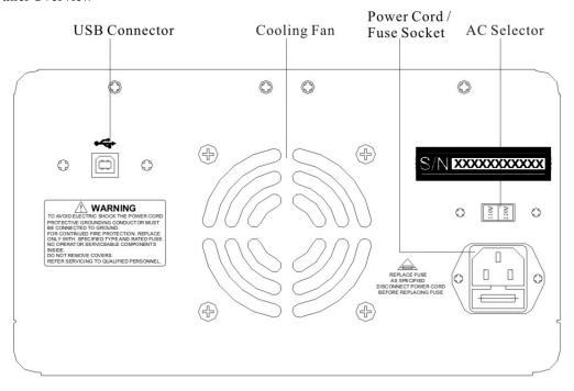
Fig.1.6-1 Rear panel of MPD-3303S/3303D/3305D
