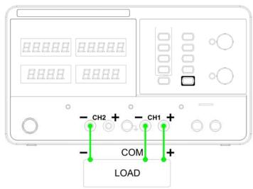
Output rating  $0\sim30\text{V}/0\sim3\text{A}$  for CH1 $\sim$ COM (I $\leq$ 3A)  $0\sim30\text{V}/0\sim5\text{A}$  for CH1 $\sim$ COM (I>3A)  $0\sim30\text{V}/0\sim3\text{A}$  for CH2 $\sim$ COM (I $\leq$ 3A)  $0\sim30\text{V}/0\sim5\text{A}$  for CH2 $\sim$ COM (I>3A)
