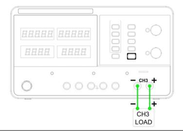
Output rating Fixed 2.5V/3.3V/5V, 3A
