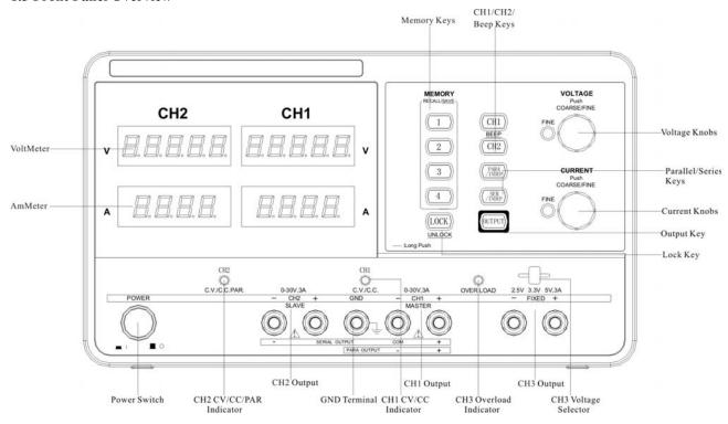
Fig.1.5-1 Front panel of MPD-3303S
