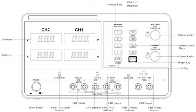
Fig.1.5-2 Front panel of MPD-3303/3305/3303C/3305C/3303D/3305D
