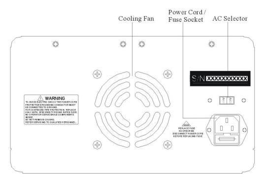
Fig.1.6-2 Rear panel of MPD3303/3305/3303C/3305C
