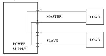
Fig. 4-5 Parallel Tracking Operation.
