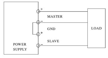
Fig. 4-4 Positive and Negative Supply.
